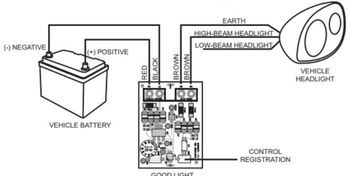
**NOTE:** Keeping Good Light's two switches, SW1 and SW2, pressed simultaneously until the LED turns off, the Fixed Code control RF transmission protocol is inverted for Rolling Code control and vice versa.
